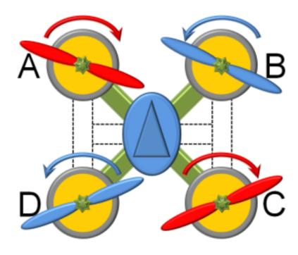
To move ahead D and C have to turn faster than A and B to increase thrust of "the back". If A and B turn faster than C and D, the craft will move backward.
