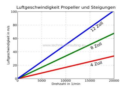
However, we need to consider that the real air speed is approximately 10% less than indicated owing to losses of streaming. The air stream generated by the rotor has to be significantly faster than the lift speed. E.g. if a lift speed of 70 km/h, i.e. 19 m/s, is meant to
