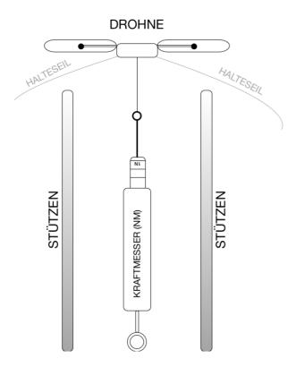
The drone rests on two poles, the stabilizing strings need to be slightly longer than the expected extension of the newtonmeter. While launching the aircraft the upward force can be directly read.
